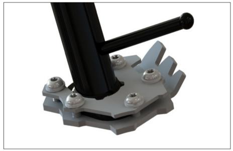
Snug tight in turn with T25 wrench but do not over-tighten to the point of distorting the top plate. Check again after first ride, then again at 100miles.
